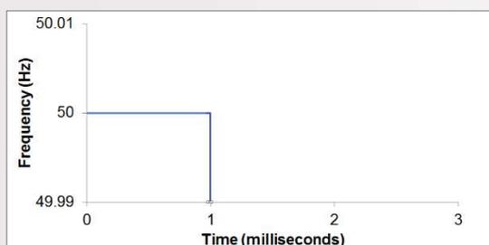
PEC generator has no inertia so frequency could change abruptly on a millisecond timescale, destabilising grid.
